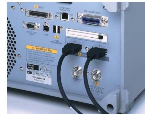
Example of Logic Probe Connection
