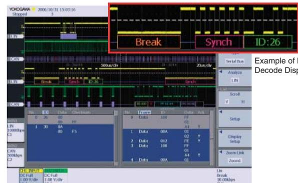
Example of simultaneous analysis and waveform (decode) display of CAN and LIN bus signals
