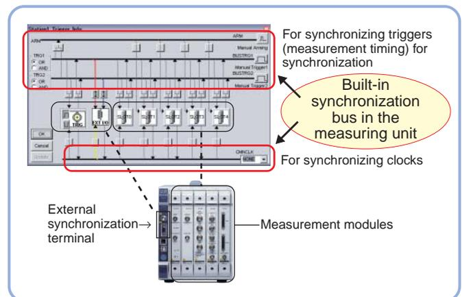
Since buses for synchronizing trigger timing and sampling clock are built into the station, there is no need to connect cables for synchronization.
