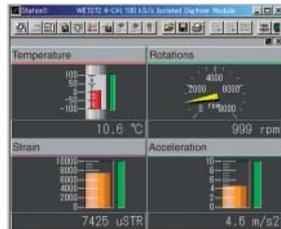
Waveforms and instantaneous values can be displayed in various styles according to your application. Two display formats are available for the different measurement methods, continuous trend display analogous to a recorder and high-speed repetitive display analogous to an oscilloscope.
