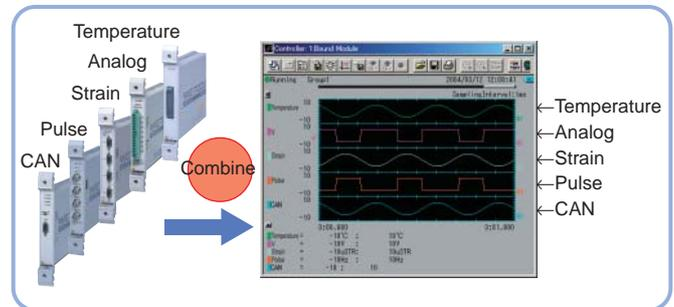
Different modules can operate as one group. Various signals such as temperature, analog, strain, pulse, and CAN can be measured simultaneously. For modules with slow sampling rate, the data is interpolated. The same number of data samples for each module is saved collectively to the same file.
