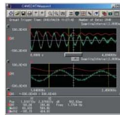
The data saved to a file can be analyzed later. Comparison by overlapping data with past data and complicated analysis using computation functions (option) are possible.
