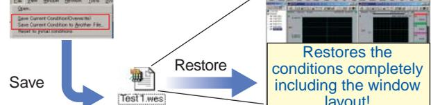
All the current conditions such as the measurement conditions and waveform display conditions, and equations of each module can be saved to an arbitrary file. Simply double-click the saved file to restore the conditions instantly. In addition, the measurement conditions of each module can be saved to separate files or to the memory in the module.
