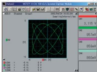
This feature is effective when evaluating the change in torque and fuel consumption rate (vertical axis) versus the number of rotations of the engine (horizontal axis) and the evaluation of DC motors using lissajous waveforms.
