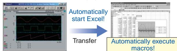
Excel is automatically started, and the current waveform data is automatically transferred to the cells on Excel. Furthermore, a specified macro can be executed automatically after the transfer.
