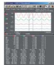
Equations can be defined using abundant functions including four arithmetic operations, trigonometric functions, differentiation, integration, digital filter, FFT, pulse width computation (duty and period). The computed result can be specified as a parameter in other equations.
