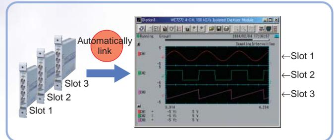
When multiple modules of the same type are inserted in adjacent slots, the modules are automatically recognized as if one module with multiple channels had been inserted. Of course, the modules can also operate independently.
