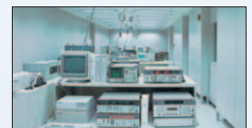
Temperature- and humidity-controlled calibration room
