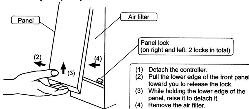
Figure 6-1 Detaching the air filter
