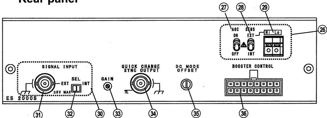
**26 Switches and connectors related to remote sensing AGC.**
