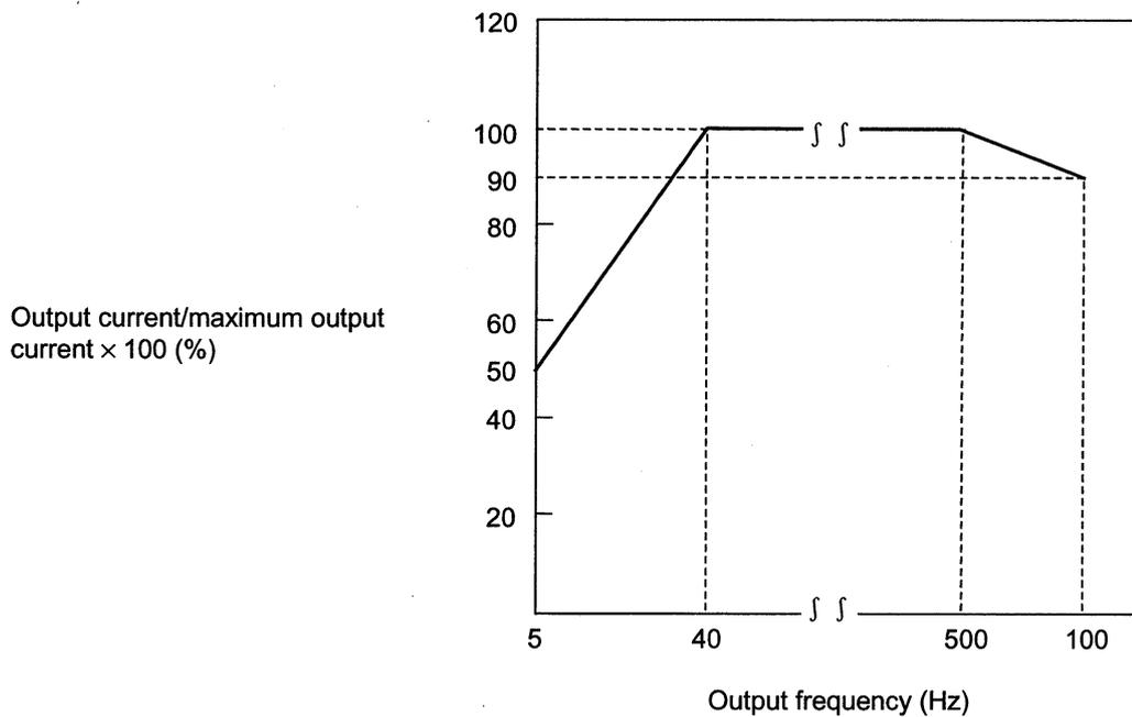
Figure 5-2 Output frequency vs. output current characteristic
