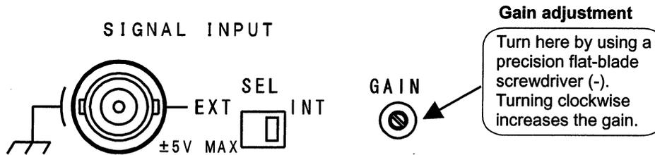
This section describes how to adjust the gain of the internal amplifier by using the measurement function of this device. To adjust the gain, follow the procedure below.
