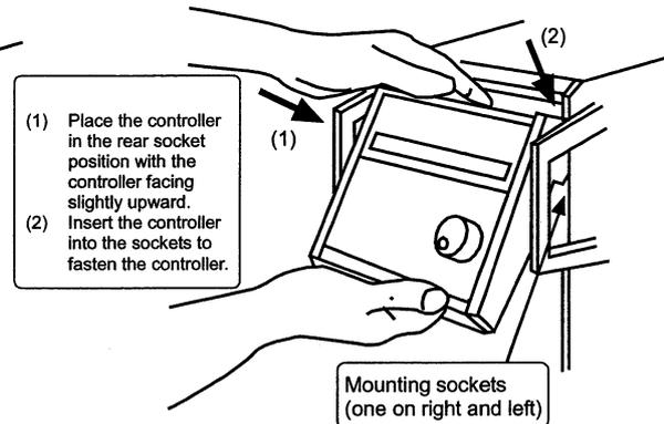
Figure 4-3 Fastening the controller while it faces upward
