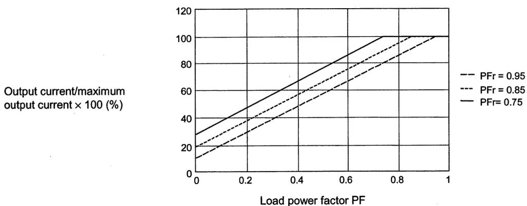
Figure 5-4 Load power factor PF vs. output current
