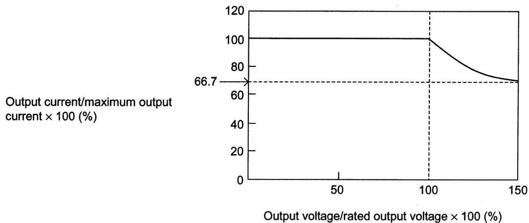
Figure 5-1 Output voltage vs. output current characteristic
