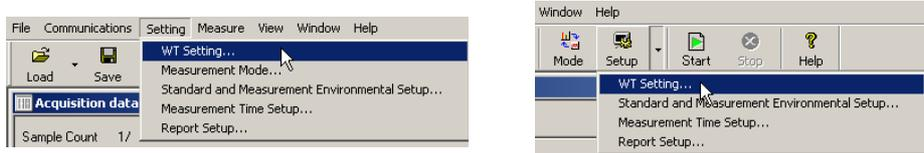
2. On the WT Setting dialog box, select the Simple Mode or Detail Mode tab.
