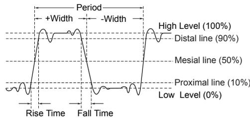
Pulse: Pulse count Adjust the measurement scope to the pulses you want to measure.
