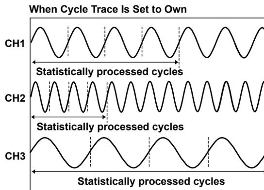
The number of cycles in the channel with the slowest cycle (CH3) is four, so statistical processing is performed on the four oldest cycles of the data for CH1 and CH2. The remaining data is not used for statistical processing.
