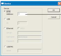
Input the GP-IB address of the instrument to be connected (0 to 30)
