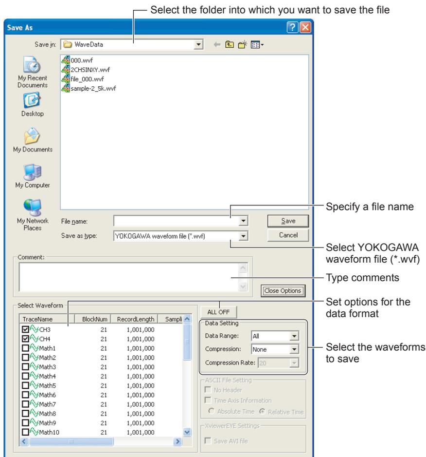
Saved WVF files can not be loaded on the measuring instrument\*.
