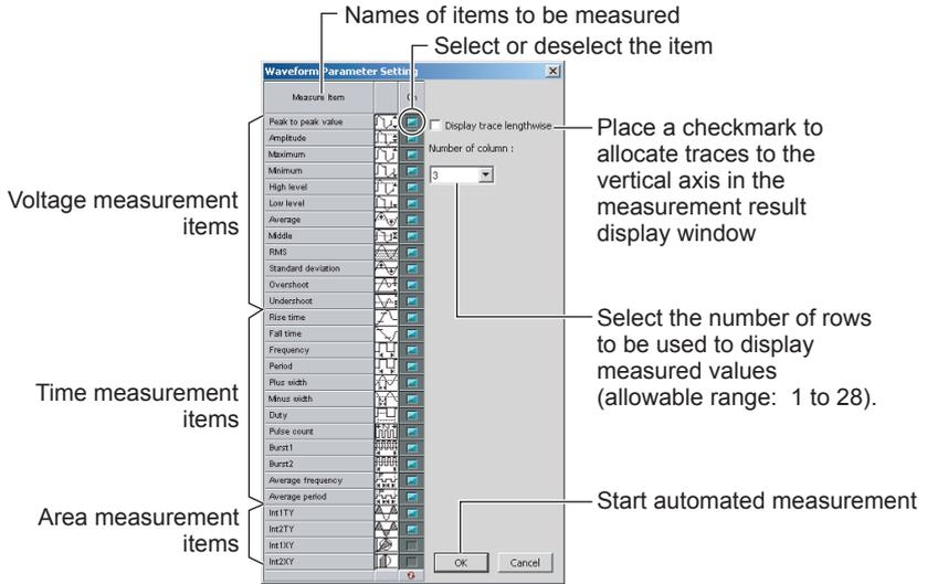
Automated measurement starts. Two vertical cursors are displayed in the main waveform display window, and the measured results of waveform parameters are displayed in the measurement results display window.
