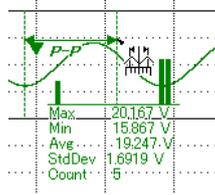
b. Double-click to display the dialog box below. You can set the measured items, the trace (waveform) to which the annotation is linked, the display format, the arrow style, and other items. The measurement range of the new cycle statistics displayed when you double-click is 2 div.
