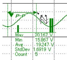
b. Double-click to display the dialog box below. You can set the measurement items, the trace (waveform) to which the annotation is linked, the display format, the arrow style, and other items. The measurement range of the new history statistics displayed when you double-click is 2 div.
