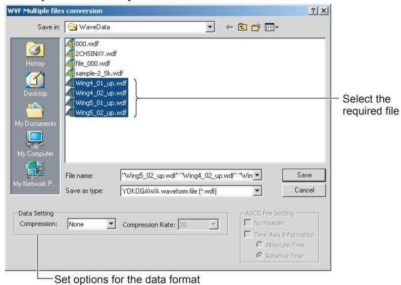
4. Select a save destination folder and click **OK**. The converted WVF files are saved in the selected folder. Converted files are only given the wvf file name extension. Converted WVF files can not be loaded on the measuring instrument.
