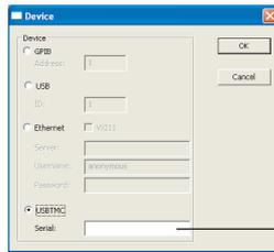
Input the serial number of the instrument to be connected (9-digit)
