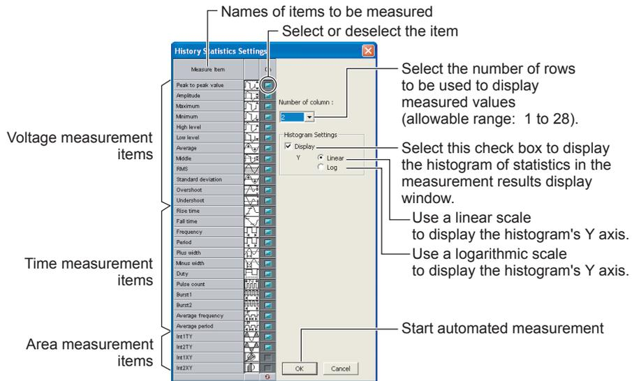
Automated measurement starts. Two vertical cursors appear in the main waveform display window, and the measured history statistics are displayed in the measurement results display window.
