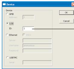
Input the USB ID number of the instrument to be connected (1 to 127)
