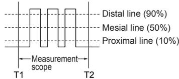
Burst1, Burst2: Burst width [s] Adjust the measurement scope to the burst widths you want to measure.
