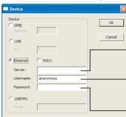
Input the IP address of the instrument to be connected
